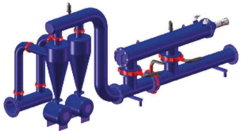
The **IPLAST IPH** series are automatic, self-cleaning filters, ideal for remote installation sites, with a water-driven self-cleaning mechanism that doesn't require an external power source for operation. With a variety of screen areas the IPH models support flow rates of up to 180 m<sup>3</sup>, down to 50 micron and inlet/outlet diameters from 4" to 8".
